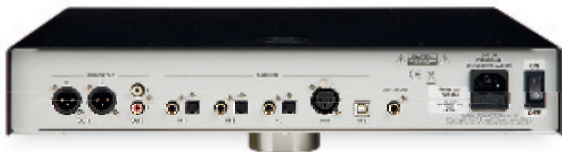
ABOVE: Balanced (XLR) and single-ended (RCA) analogue outs are joined by AES/EBU (XLR) and USB digital inputs alongside three Toslink optical and three coaxial S/PDIF
