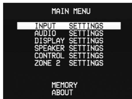
The **MAIN MENU** gives access to a series of menus which allow you to customize different aspects of the operation of the SP32 using the on-screen display.
